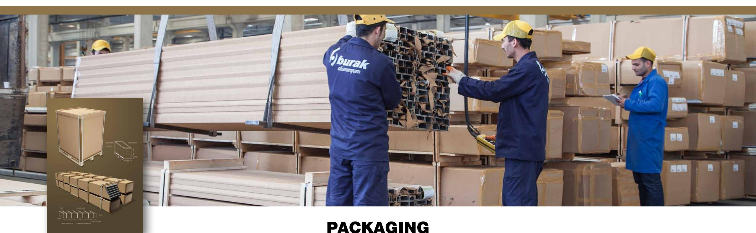
Aluminium profiles need to be maintained safe from against environmental factors during transfer, shipment or stock. For the protection of aluminium extrusion profile surfaces, they need to be taped and film covered, bulk case packaging with nylon and craft paper; and they also need separate packaging so that they can be carried by forklifts, cranes or trucks in
